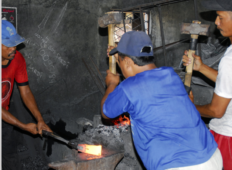
Figure 6.7d Striking the billet while it's hot at Meteor workshop in Solo, Java, Indonesia (photograph by Carol Ventura, 2007).
