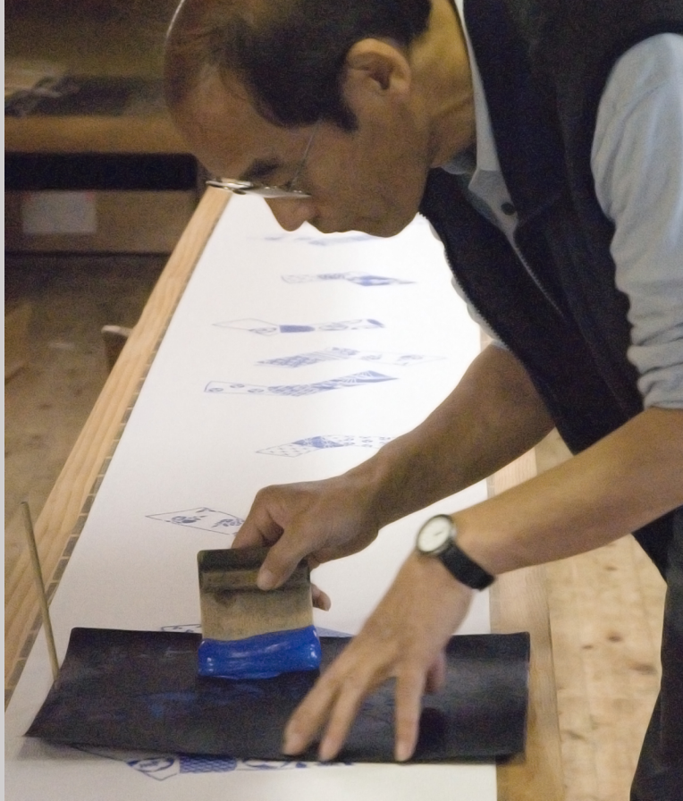
Figure 6.24d Printing blue resist onto cloth with a katazome stencil, Kuriyama Koubou, Kyoto, Japan (photograph by Carol Ventura, 2006).
