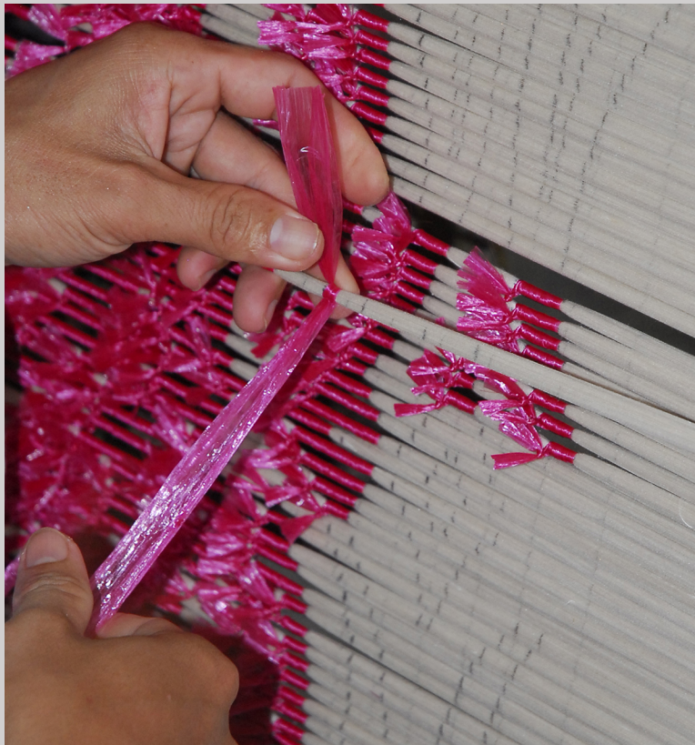
Figure 6.5b Following a graphed pattern to precisely mark weft bundles at Pertenunan Berdikari Handwoven Cloth Factory in Singaraja, Bali, Indonesia (photograph by Carol Ventura, 2007).
