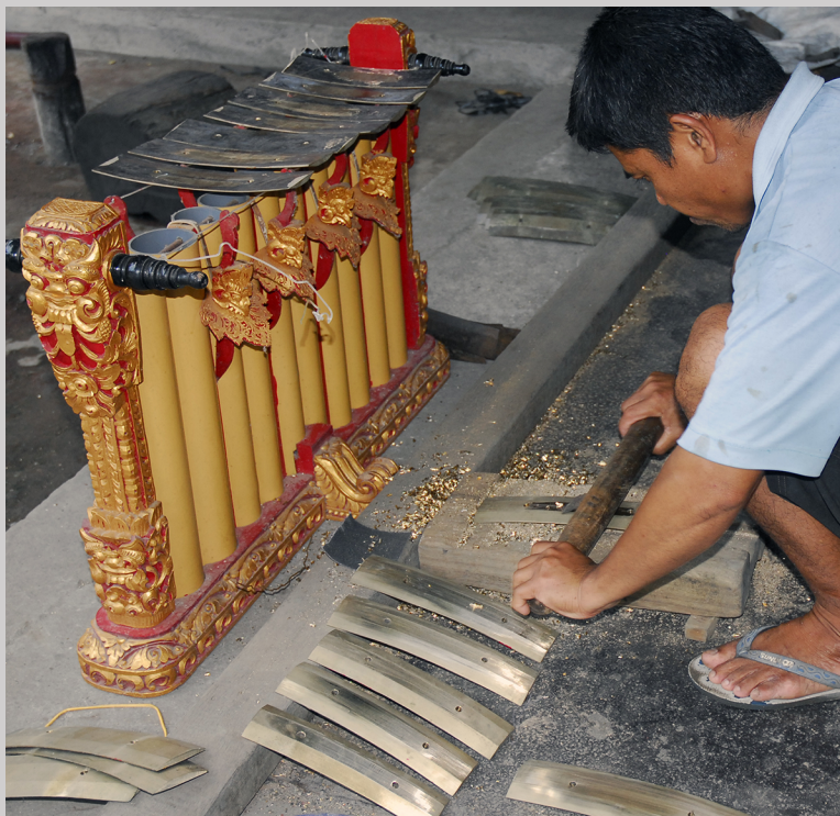
Figure 6.9f Fine tuning brass gangsa keys at Sidha Karya, Banjar, Bali, Indonesia (photograph by Carol Ventura, 2007).
