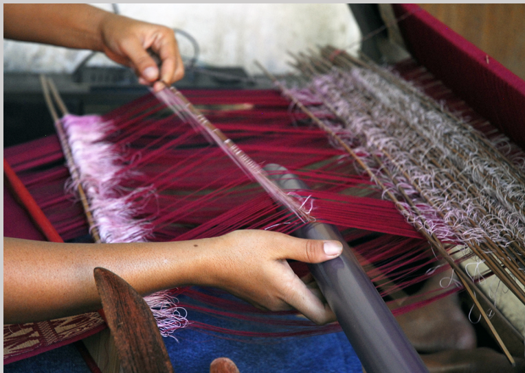
Figure 6.4d The shed is changed again by releasing the tension by moving slightly forward while pulling up the next string heddle rod (photographs by Carol Ventura, 2007).
