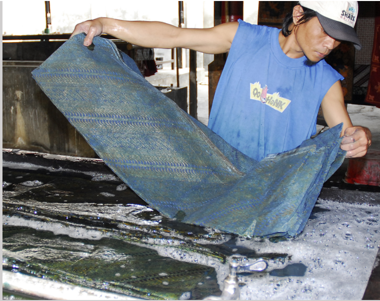
Figure 6.2k Dyeing waxed cloth in a rectangular shallow vat at Batik Plentong, Yogyakarta, Java, Indonesia (photograph by Carol Ventura, 2007).
