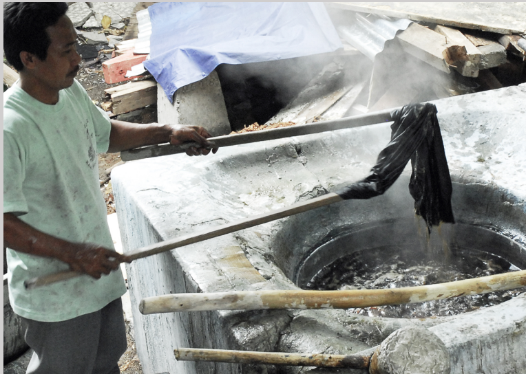
Figure 6.2n Removing wax from cloth in boiling water at Batik Indah, Yogyakarta, Java, Indonesia (photograph by Carol Ventura, 2007).
