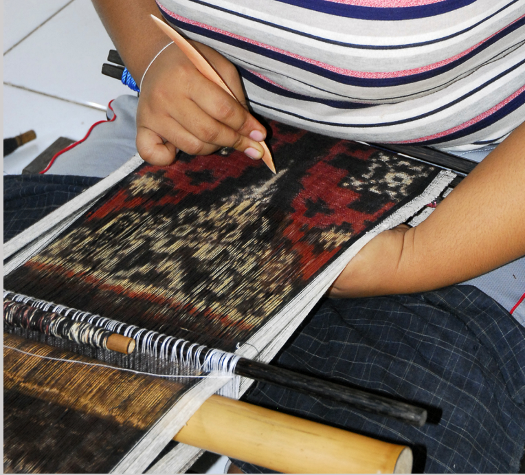
Figure 6.5g Using a pick to adjust the warp and weft while weaving double ikat geringsing on a body-tensioned loom in Tenganan, Bali (photograph by Carol Ventura, 2007).
