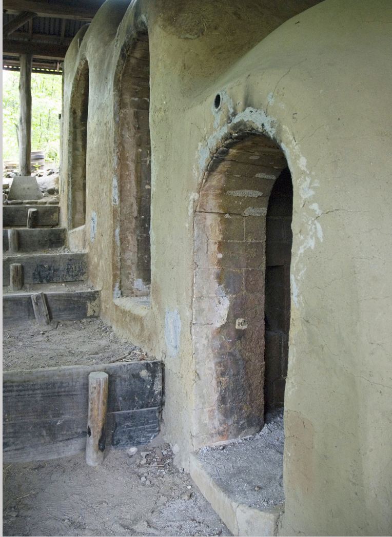
Figure 6.16b Noborigama kiln side doors at the Shigaraki Ceramic Cultural Park, Japan (photograph by Carol Ventura, 2006).
