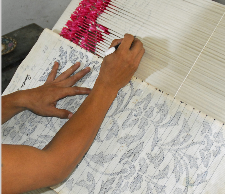
Figure 6.5b Following a graphed pattern to precisely mark weft bundles at Pertenunan Berdikari Handwoven Cloth Factory in Singaraja, Bali, Indonesia (photograph by Carol Ventura, 2007).
