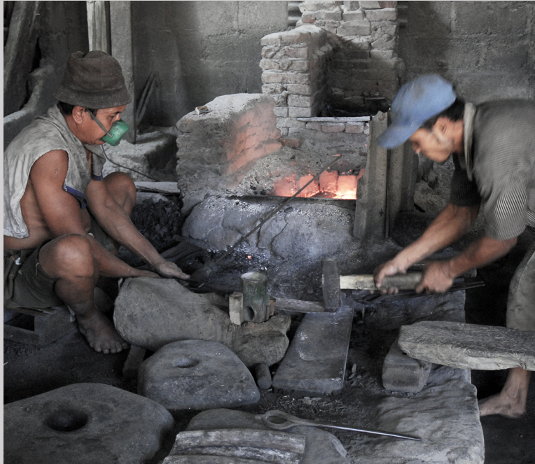
Figure 6.9d Hammering a hot brass gangsa key at Gong Yudha, Tihingan, Bali, Indonesia (photograph by Carol Ventura, 2007).
