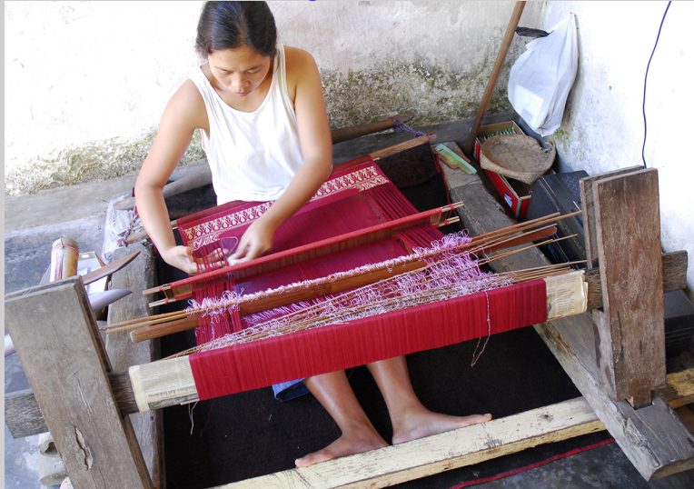
Figure 6.4b Supplementary metallic weft is inserted in Sideman, Bali, Indonesia (photograph by Carol Ventura, 2007).
