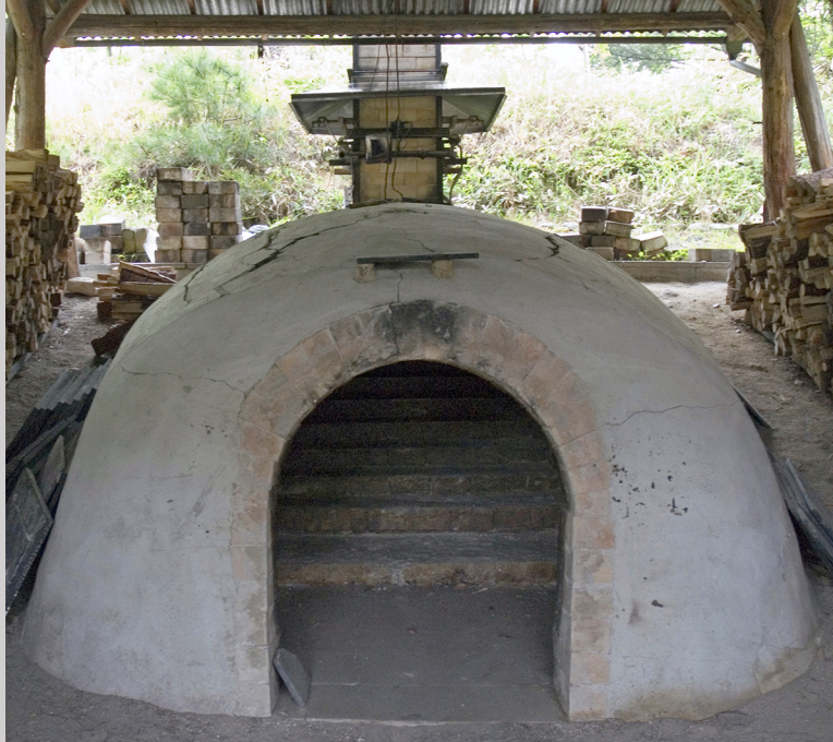
Figure 6.14a Outside an anagama kiln looking towards the chimney, Shigaraki Ceramic Cultural Park, Japan (photograph by Carol Ventura, 2006).
