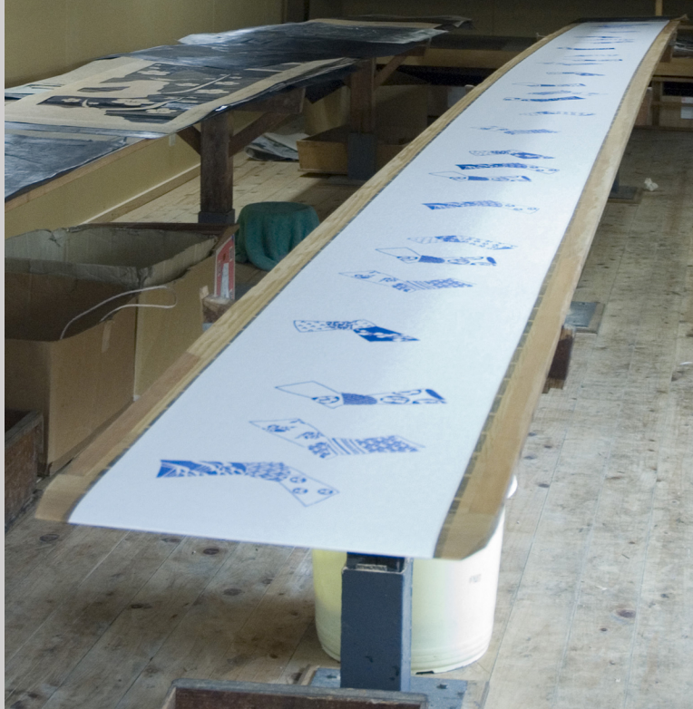
Figure 6.24c Preshrunk silk stretched onto a board, Kuriyama Koubou, Kyoto, Japan (photograph by Carol Ventura, 2006).
