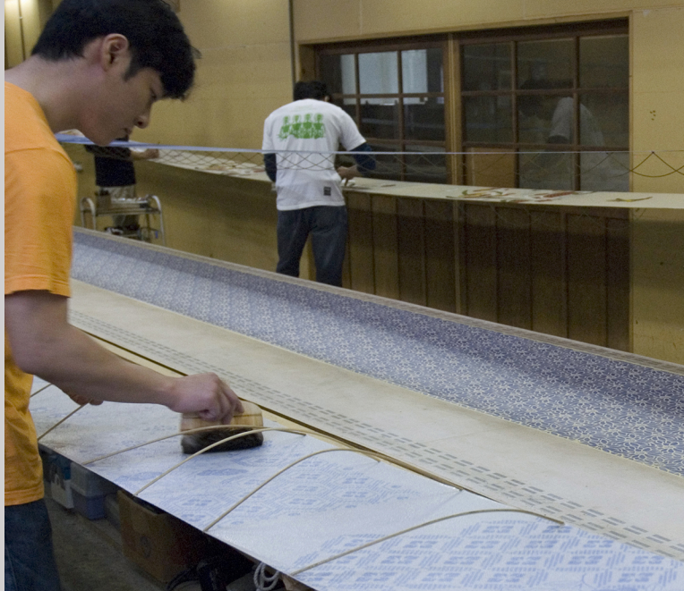
Figure 6.24i Sizing is brushed onto stretched, resist stenciled silk, Kuriyama Koubou, Kyoto, Japan (photograph by Carol Ventura, 2006).
