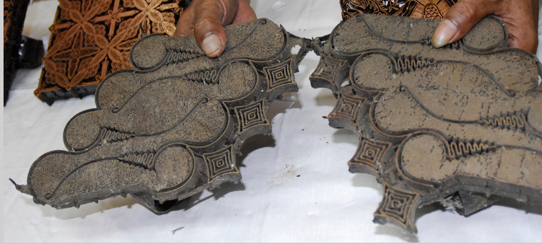
Figure 6.2f Pair of metal caps used to stamp the same pattern on the front and back of thick cloth. The wire sticking out on the far left of the left cap helps to correctly position the cap on the cloth at Batik Indah in Yogyakarta, Java, Indonesia (photograph by Carol Ventura, 2007).
