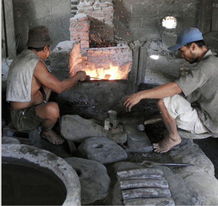
Figure 6.9c Heating a gangsa key at Gong Yudha, Tihingan, Bali, Indonesia (photograph by Carol Ventura, 2007).
