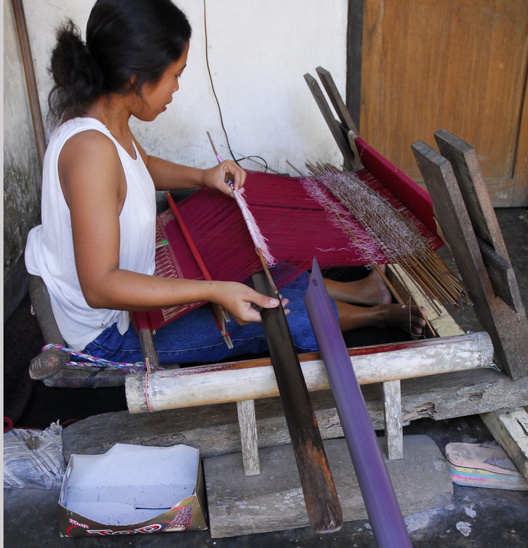
Figure 6.4c The shed is changed by pulling up a string heddle rod and then the beater is inserted to help open the shed in Sideman, Bali, Indonesia (photograph by Carol Ventura, 2007).
