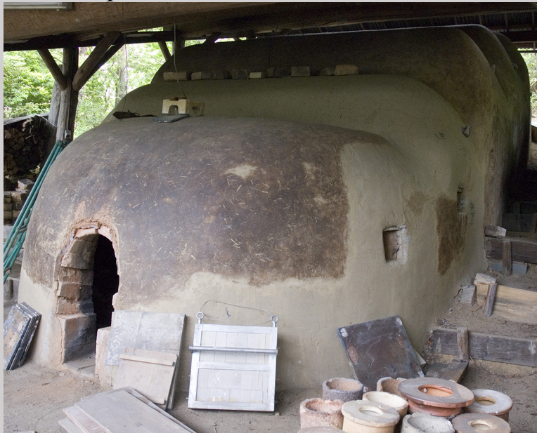
Figure 6.16a Wood fired Noborigama kiln at the Shigaraki Ceramic Cultural Park, Japan (photograph by Carol Ventura, 2006).
