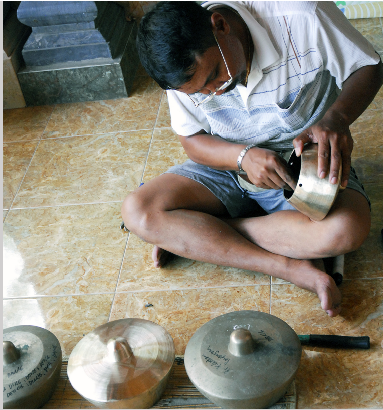
Figure 6.9g Fine tuning brass bonangs (small metal gongs) at Sidha Karya, Banjar, Bali, Indonesia (photograph by Carol Ventura, 2007).
