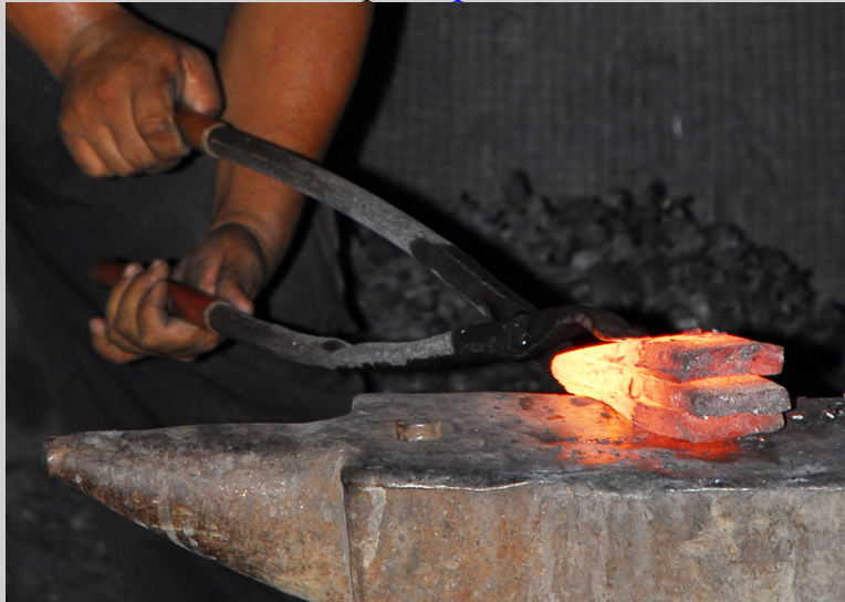
Figure 6.7c Partial forge welded billet at Meteor workshop in Solo, Java, Indonesia (photograph by Carol Ventura, 2007).
