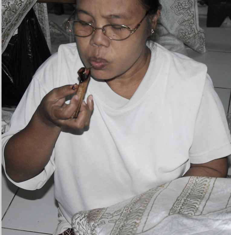
Figure 6.2d Unclogging a canting tool by blowing into the tube at Galeri Batik Kuno Damar Hadi, Surakarta, Java, Indonesia (photograph by Carol Ventura, 2007).
