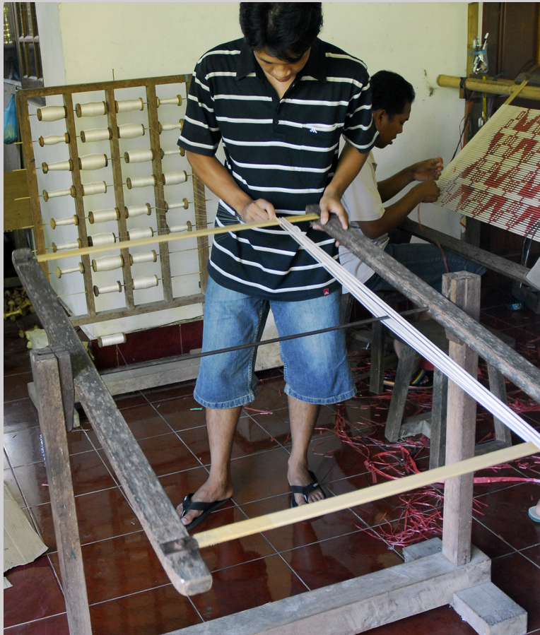
Figure 6.5a Measuring weft on a rotating frame at Pelangi in Sideman, Bali, Indonesia (photograph by Carol Ventura, 2007).
